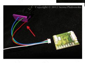
3. Connect the wires to the OBD2 socket
