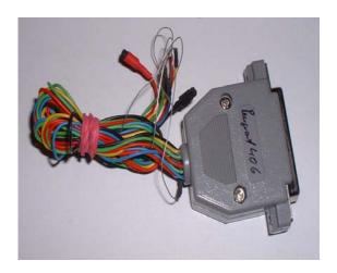
The blue cable comes from the 4 cables that belong together, the green from the 2 data cables that belong together. The green marked pins haver to be connected together.
