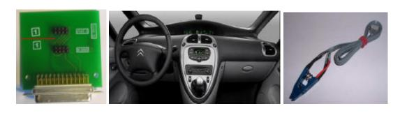
Eeprom 95020 in cluster must be desoldered and programmed to 0.
