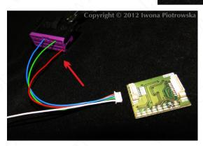
3. Connect wires to the OBD2 socket
