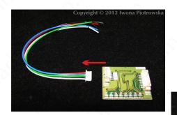
Disconnect plug with wires from
