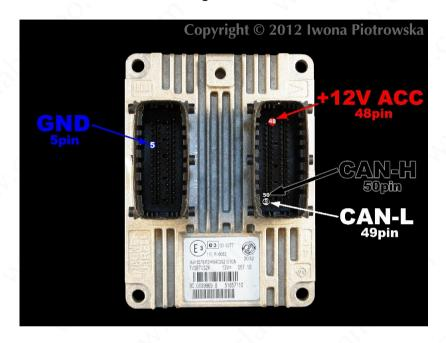
GND 6 pin +12V ACC 48 pin Can H 50 pin Can L 49 pin
