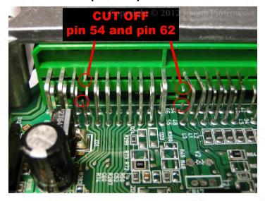
Before connecting the emulator, it must be precisely insulated with insulation tape
