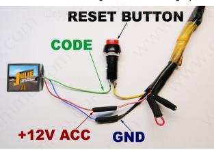
You connect code line by pressing the RESET button. In order to start the car you firstly need to press and hold the RESET button, then turn the ignition and then release the RESET button. Now you can start the engine.
