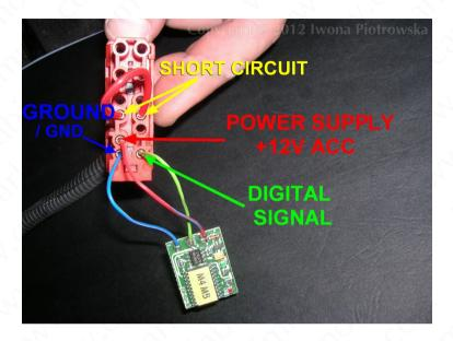
After correctly connecting the emulator, SRS/AIRBAG fault on instrument cluster goes off without necessity to delete the code of faults.
